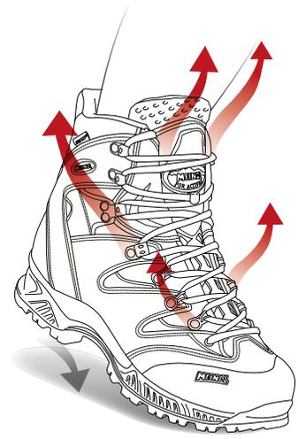
The entire tongue is a combination of 3D mesh and a permanently shock-absorbing, reticulated, perforated sponge. This works like a pump. In order to achieve an anatomical shape, a micro-fleece stabilizer is stitched onto the tongue. To fix it in place, a Velcro tab is used at the front of the boot and at the edge of the tongue.
