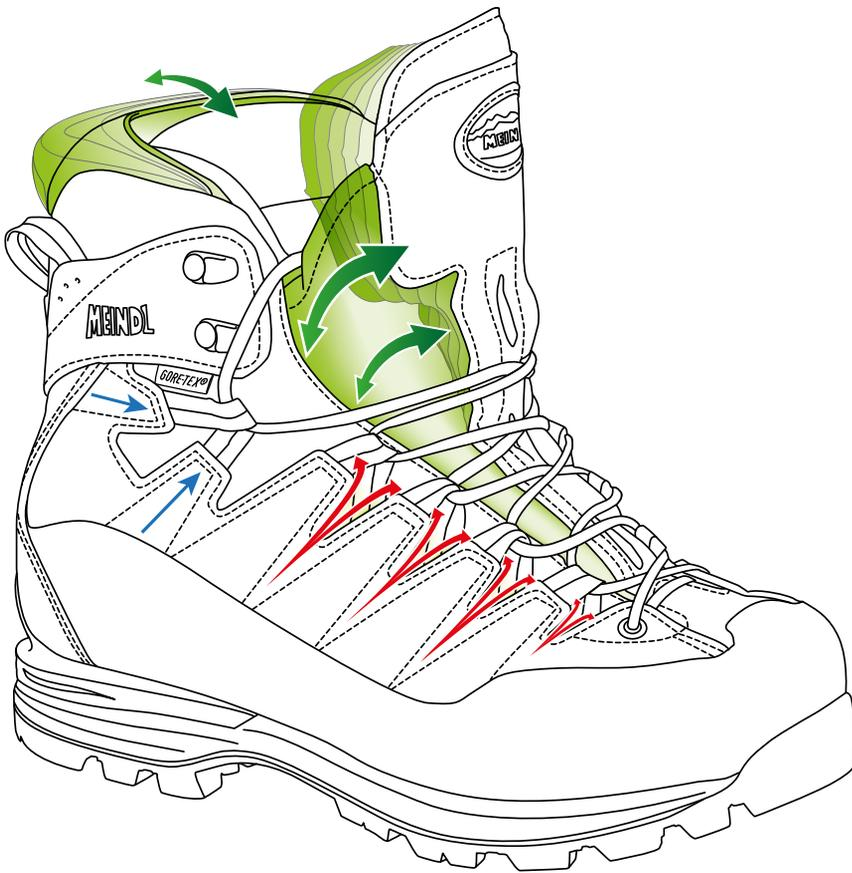
The upper is softer and more flexible towards the top, enabling careful walking, climbing and accordingly a safe crampon technique. The soft edge of the upper prevents uncomfortable pressure and sore areas.
